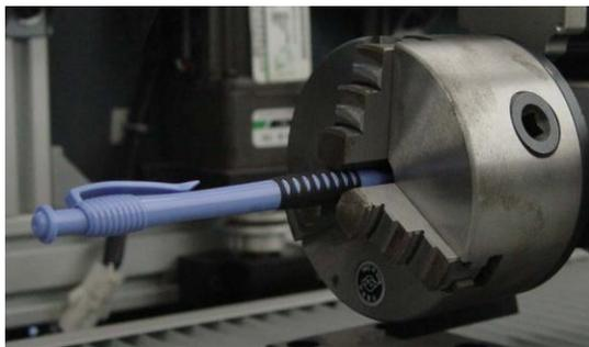
Rotary clamp B (with a chuck)
