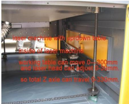
laser machine with up/down table
